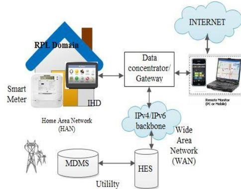
Figure 3: IoT enabled Smart Metering Architecture
