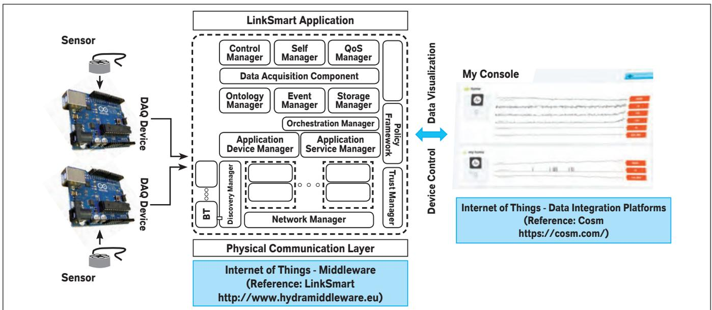
Figure 3: A High Level Diagram of a Data Acquisition Architecture Involving the Technologies Mentioned in the Article
